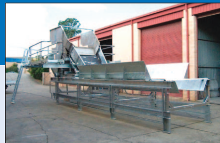
The assembled Newstan dewatering system before delivery.
