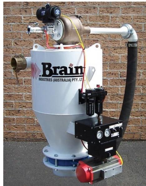
**OPERATION** - Automatically controlled by pneumatic timers pre-set to achieve an optimum fill and discharge cycle with manual override capability.
