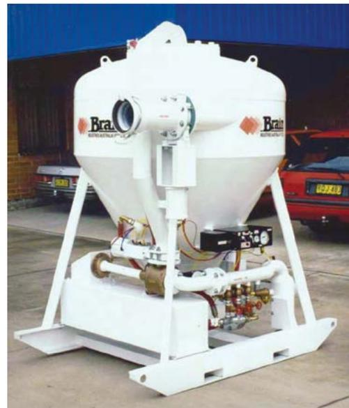
**OPERATION** - Automatically controlled by pneumatic timers pre-set to achieve an optimum fill and discharge cycle with manual override capability.
