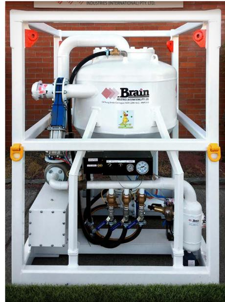
**OPERATION** - Automatically controlled by pneumatic timers pre-set to achieve an optimum fill and discharge cycle with manual override capability.
